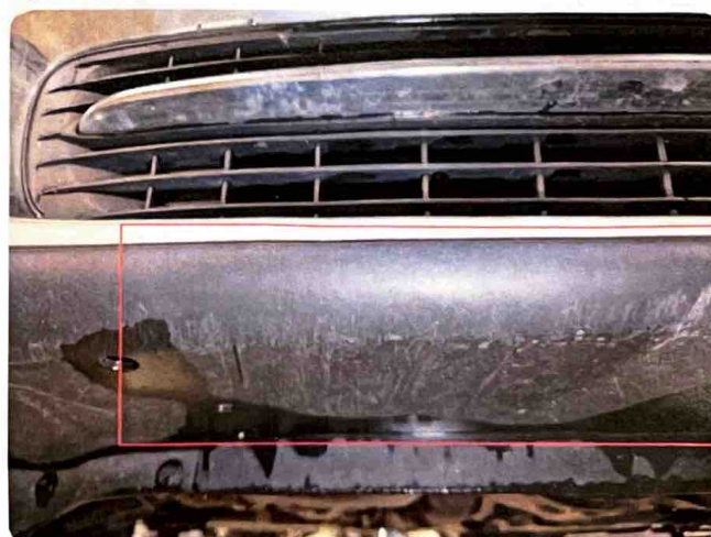
3.13 Skrubbskader underkant Noe skrubbskader underside frontfanger
