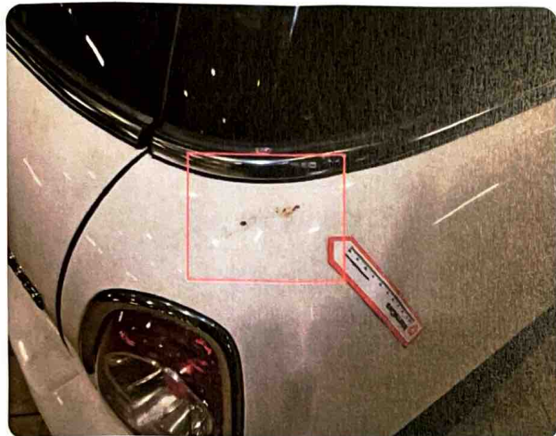
3.7 Rust Rust h-bakskjerm.
